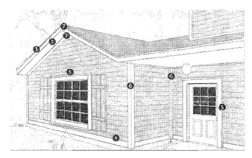
**<u>1. Fascia:</u>** A horizontal board of vertical face, usually below the edge of the roof and attached to the roof rafter tails. These boards are usually 6" - 8" wide.
